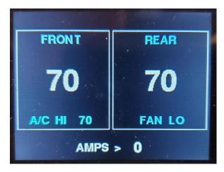
These frames show the current temperature in the middle of frame, and the current mode and set point for the front / rear at the bottom of frame.
