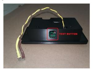
1) Activate the calibration mode by momentarily pressing the TEST BUTTON on top of the TS display.
