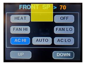
The yellow highlighted area at the top center shows a touch sensitive area that allows you to toggle between the front mode page and the rear mode page.
