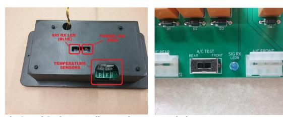
The OP and CM have a small LED indicator to signal when it receives a communications packet. Information packets are exchanged at least every ten seconds or immediately if a temperature, set point, or status changes. The blue (or red) LED on the OP or the SIG RX LED on the CM blink whenever they receive a packet.
